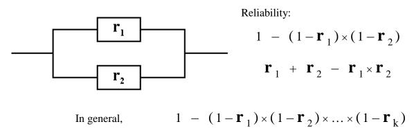
**7.** Compute the reliability of the following system of independent components (the numbers represent the reliability of each component):
